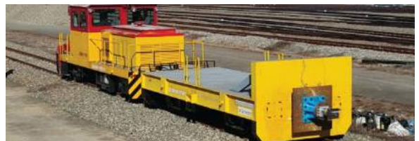
Dynamic testing of Category C buffer, KRRI
