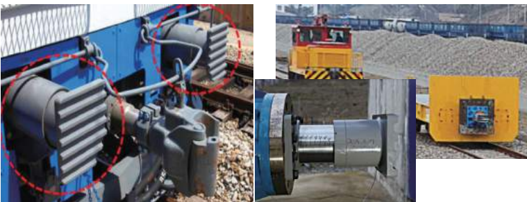
Dynamic testing of Electric railway buffer, KRRI
