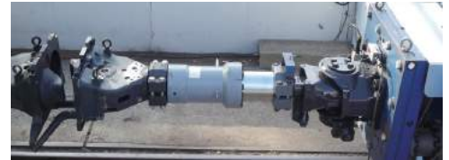
Dynamic testing of buffer, TÜV SÜD
